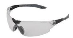
Extremely light and comfortable safety glasses with modern styling. Temples have soft tips, soft black aerated nose bridge ensures comfortable wear. Clear lens are anti-fogging, anti-scratching and resistant to low-energy shocks (up to 45 m/s) at extreme temperatures ( $-5 ^{\circ}\text{C} - +55 ^{\circ}\text{C}$ ).
