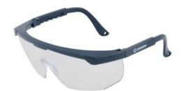
Safety glasses with dark blue nylon frame and temples. This glasses perfectly fit to every user thanks to adjustable lenght of temples. Large clear polycarbonate lens which are made from one piece protect against UV radiation and are resistant to low-energy shocks (up to 45 m/s) at extreme temperatures (-5°C - +55°C). They provide maximum protection and extremely wide field of vision.
